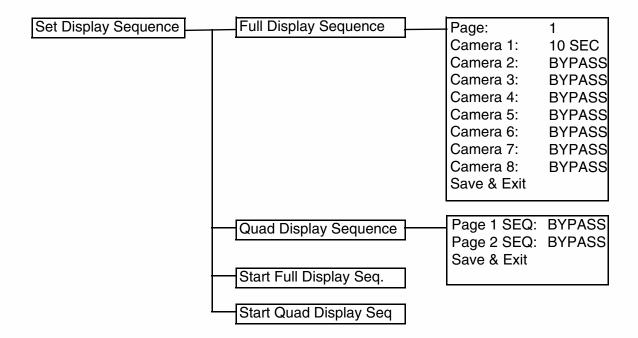
**NOTE**: The number of cameras displayed on submenus will change based on the Model of DVR: 4, 8 or 16 Cameras are available.
